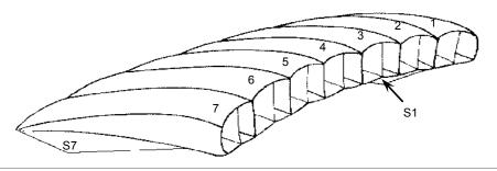
The Apex BASE *UltraLite* canopies are built using new technologically advanced fabric that has the same strength as traditional 0-3 fabric but is less bulky. We use the same tape configuration as found on the FLiK LV and FOX LV to reduce pack volume and weight while maintaining the structural integrity required on a single parachute BASE system. The *UltraLite* has the same
